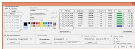
Figure 2(a): Typical SimMet® software wizard to assist users to model their experimental designs, define a data analysis pipeline that includes peak detection and picking, RT alignment, MS and MS/MS database search and statistical analysis.
