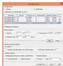
Figure 6: SimMet® software GUI for averaging MS or MS/MS scans. Filters based on scan numbers, retention time, precursor m/z are provided in order to facilitate easy selection of the target scans.
