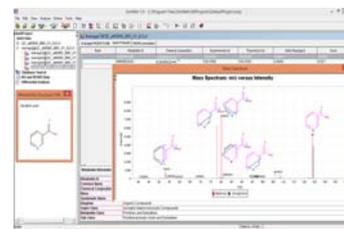
Figure 7: Typical SimMet® software result page displaying accurate identification of nicotinic acid as the compound X.
