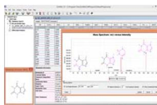
Figure 5(a): Typical SimMet® software result page displaying accurate identification of caffeine as the compound eluted at 1.9257 min of LC timescale. The result page displays identified compounds, structures, metabolite information such as ID number of public databases, common name, other database links besides annotated MS/MS spectrum with matched ions.
